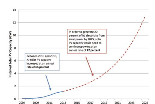
Figure 6. New Jersey Can Generate 20 Percent of Its Electricity from Solar Power by 202574
